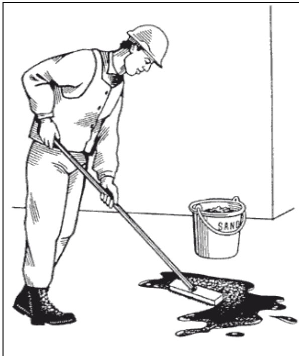
Figure 6. Clean up spilt oil or grease
